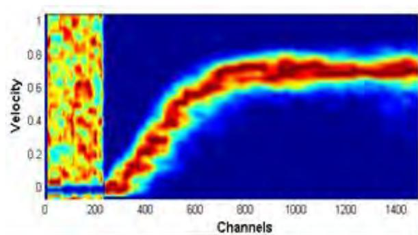
**Fig. 10** Velocity profile of Heinz ketchup, (flow rate of 56 L/min)
