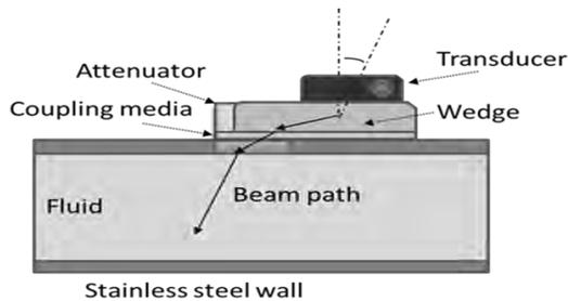
Fig. 4 Schematic of the developed non-invasive sensor technology
