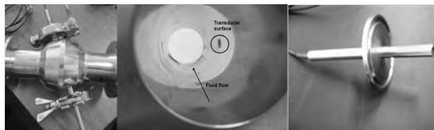
Fig. 3 Delay line pencil type transducer
