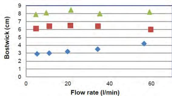
**Fig. 9** Single point measurements of ketchup with Bostwick consistometer at different flow rates
