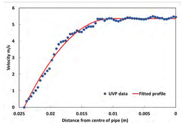
**Fig. 14** Measured and fitted velocity profiles for a 4.6% waste water sludge
