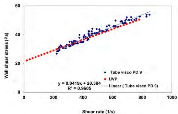
**Fig. 15** Sludge rheology comparison between tube viscometry and UVP+PD for 4.6% w/w wastewater
