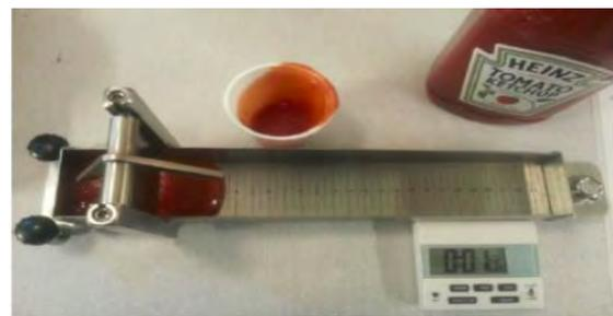
**Fig. 8** Bostwick Consistometer
