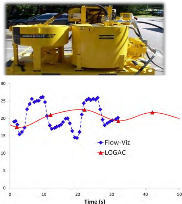
**Fig. 12** Grouting application with mixer setup Variation in flow rate measured with Flow-Viz and Logac systems
