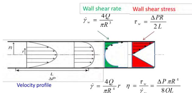
Fig. 2 Tube viscometer concept
