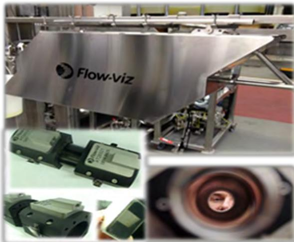
**Fig. 7** The industrially approved sensor unit featuring the unique custom made non-invasive transducer assembly.
