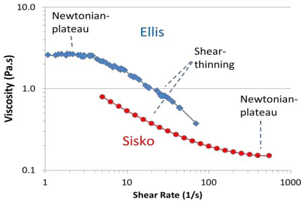
**Fig. 6** Flow curve – shear thinning fluids with Newtonian plateaus.
