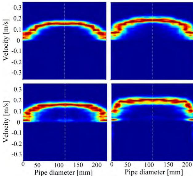
**Fig. 13** Velocity profiles of different cement grout concentrations
